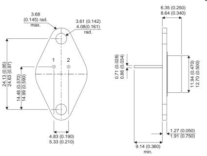
Bipolar PNP Device in a Hermetically sealed TO66 Metal Package.
